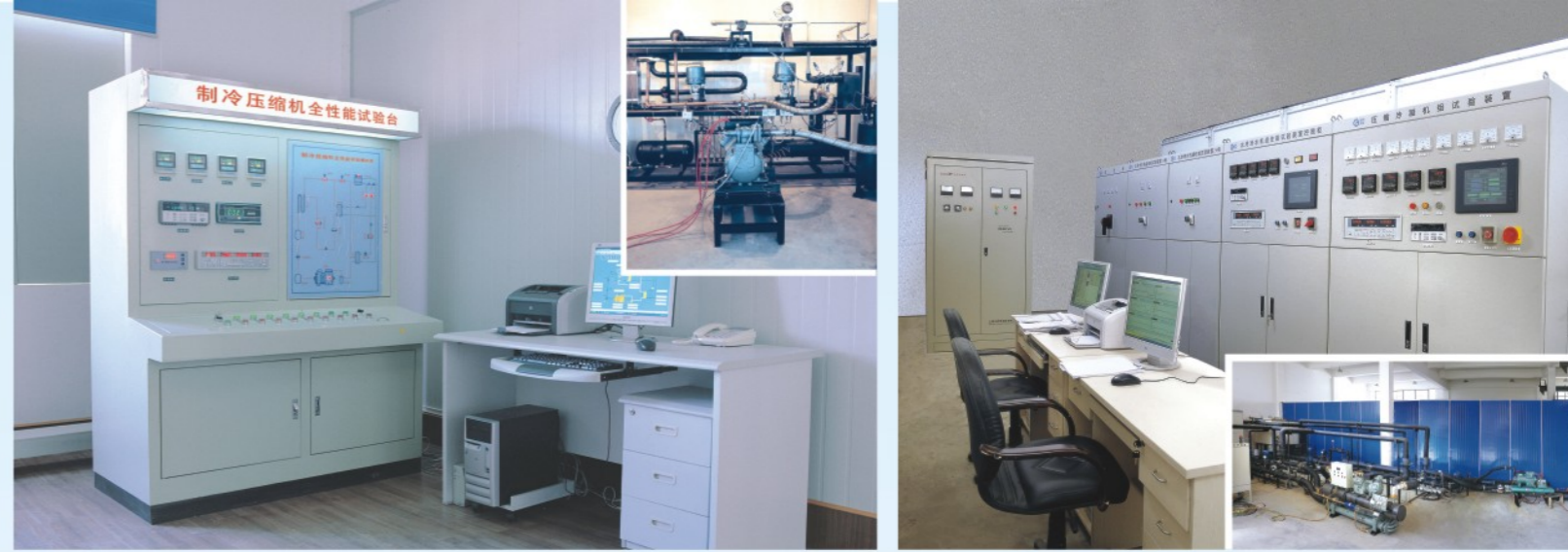
全电脑冷水机组、制冷压缩冷凝机组性能检测设备 Full-computer controlled performance inspection device of water-chilling unit and refrigerant compressor condensing unit
