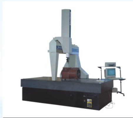
美国“Giddings & Lewis”三坐标（CNC）测量仪 Tri-coordinate CNC Measuring Machine from US Giddings & Lewis
